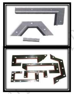
• Aluminium Strip + Polyurethane Lip: These Wipers have a basic Aluminium Strip encapsulating a high quality PU LIP, which provides excellent Slideway Wiping Capacity. They are available in five sizes out which three provide Lip protection from Hot Chips (They have frame overhand on the Lip). The aluminium strip (Frame) can be easily drilled to suit your needs. These Wipers are available in stock lengths of 500 mm to 1000 mm.
